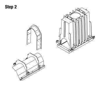
After the channel outline is removed from the catch basin, cut the inlet adapter to the height of the hole in the basin. Secure the inlet adapter to the basin using the hardware provided. Be sure to use silicone caulk or construction adhesive to seal the adaptor to the basin.
