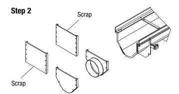
At this time attach the frame end piece with the thumb screws.
