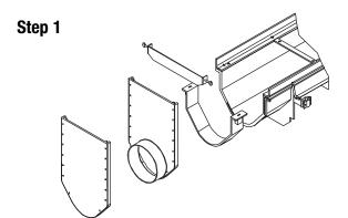
Attach end outlet or end cap with provided hardware to the channel.
