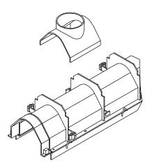
Cut out hole with hole saw that matches inside diameter of outlet.
