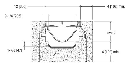
Local Codes and/or Engineer Specified concrete encasement and reinforcing based upon application suggested.
